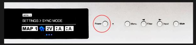
After selection is completed, wait for about 8 seconds or press the POWER button to return to the first screen.
