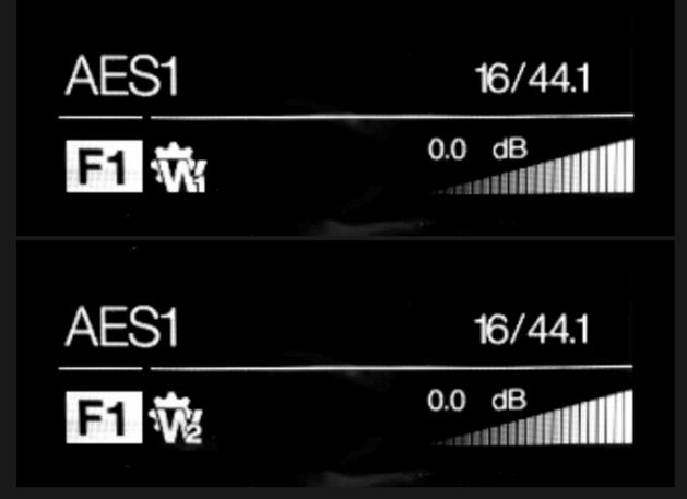
To confirm proper operation, the Word Clock Group 1 icon (W1) should appear for 44.1 kHz content. Word Clock Group 2 icon (W2) should appear for 48 kHz base content. It should change automatically on the DAC.
