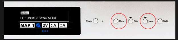
On the SETTINGS screen, press the right > button to select SYNC MODE and press the MENU button to save setting.
